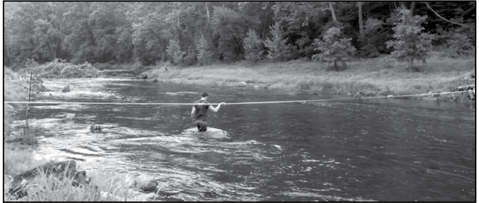
Mapping the channel for discharge at the Hughesville dam removal site.
