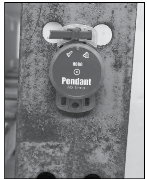
Picture of a HOBO bluetooth pendant that takes temperature readings every five minutes.
